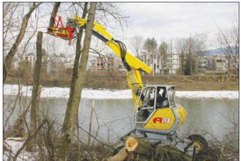
A versatile tool – mulching, or safely removing the tops of trees in town; as well as harvesting, the Menzi can do everything you would expect of an excavator.
